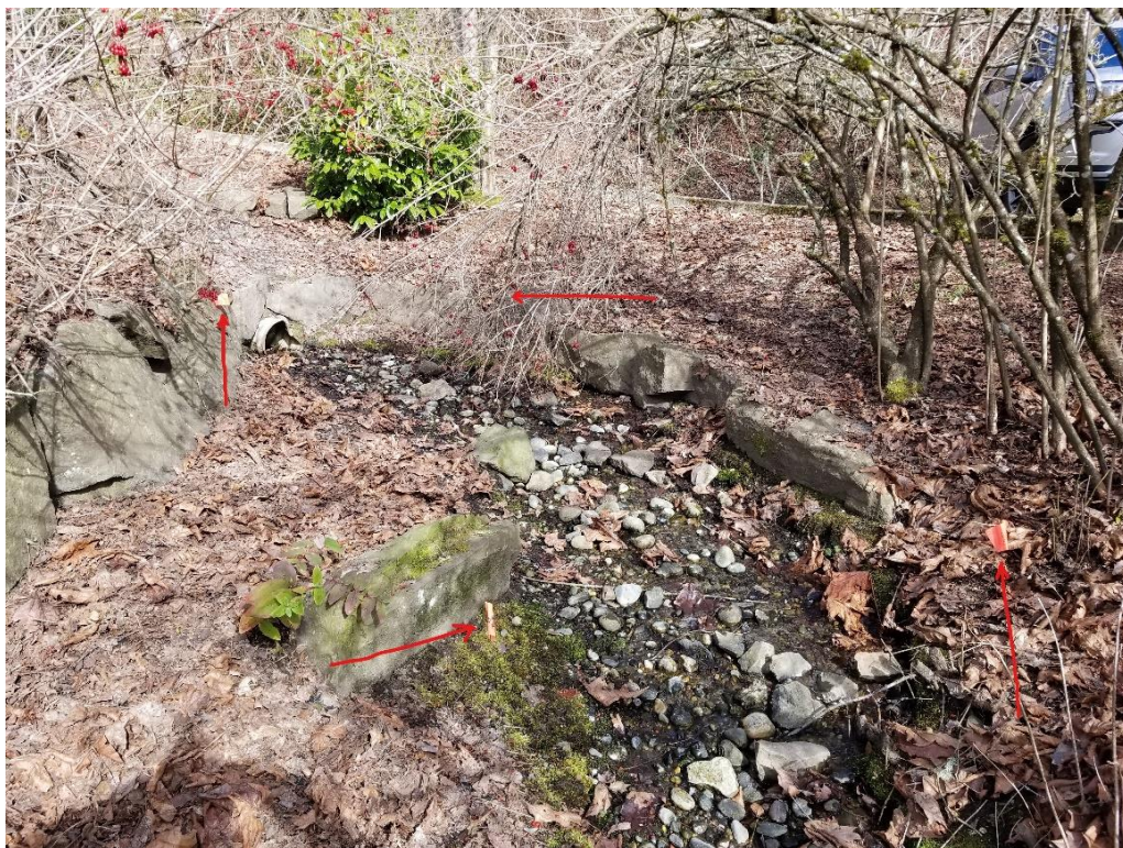
Photo 12—Delineated OHWM below the driveway, facing north. Red arrows show location of pin flags.
